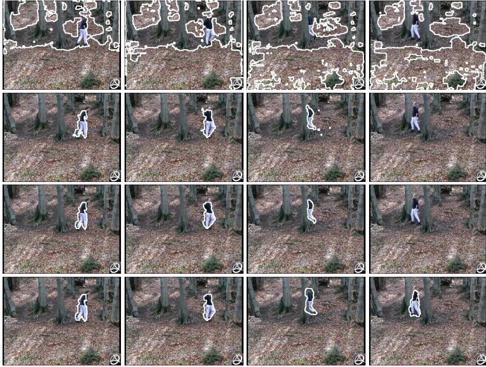
Figure 3: Tracking results for person walking in busy background. Row (A) region competition (7) without shape; row (B) fixative photometric model (5) without shape; row (C) as for (B) but with shape prior ( \lambda_\psi \neq 0 ); row (D) as for (C) but updating the fixative photometric model from frame to frame. Bootstrap from frame 10. Data from [13].
