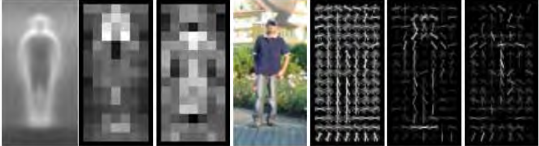
Figure 2.16: The HOG feature for human detection, adapted from [27].
