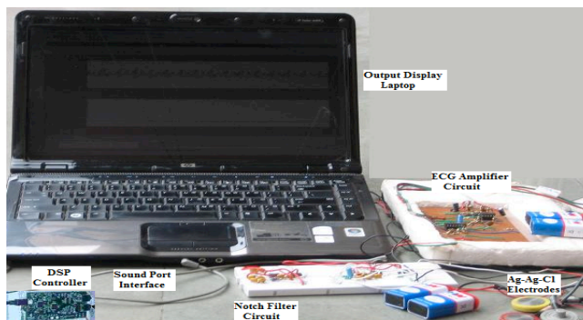
Fig. 1. Experimental set up for dsPIC DSC based System for acquisition of ECG Signals on a Computer
