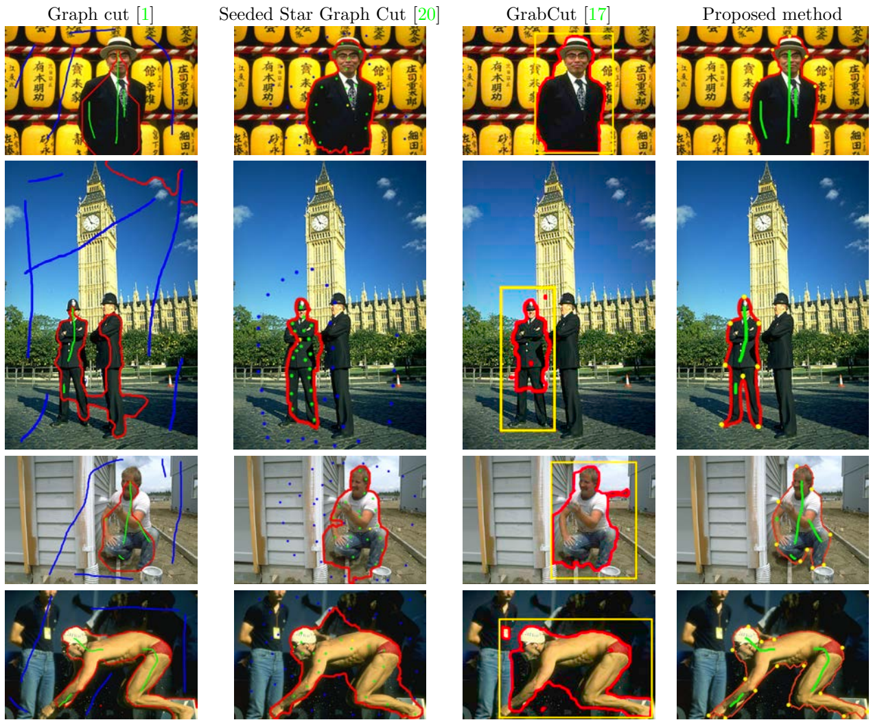
Figure 6. Segmenting human from complex scenes. From left: Original Image, Graph cut [1], Seeded Star Graph Cut [20], GrabCut [17], and proposed method. Red curve shows the segmentation result, blue for the background strokes, green for foreground strokes, and yellow for star point and the initial window of the Grabcut.
