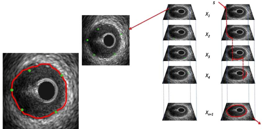
Figure 5. Example of 3D graph traversal. The stack of images on the right show how the graph is constructed out of a number of layers corresponding to the number of user points  $n + 1$ . The algorithm finds the shortest path through the layers, minimizing the costs of edges, boundaries, and distance from user points. The final result of the segmentation is shown on the left.
